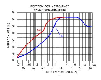
This EMI / RFI filter features a very small mechanical package. Even with this small size the common mode insertion loss and differential loss more than is available in other similarly sized packages.
